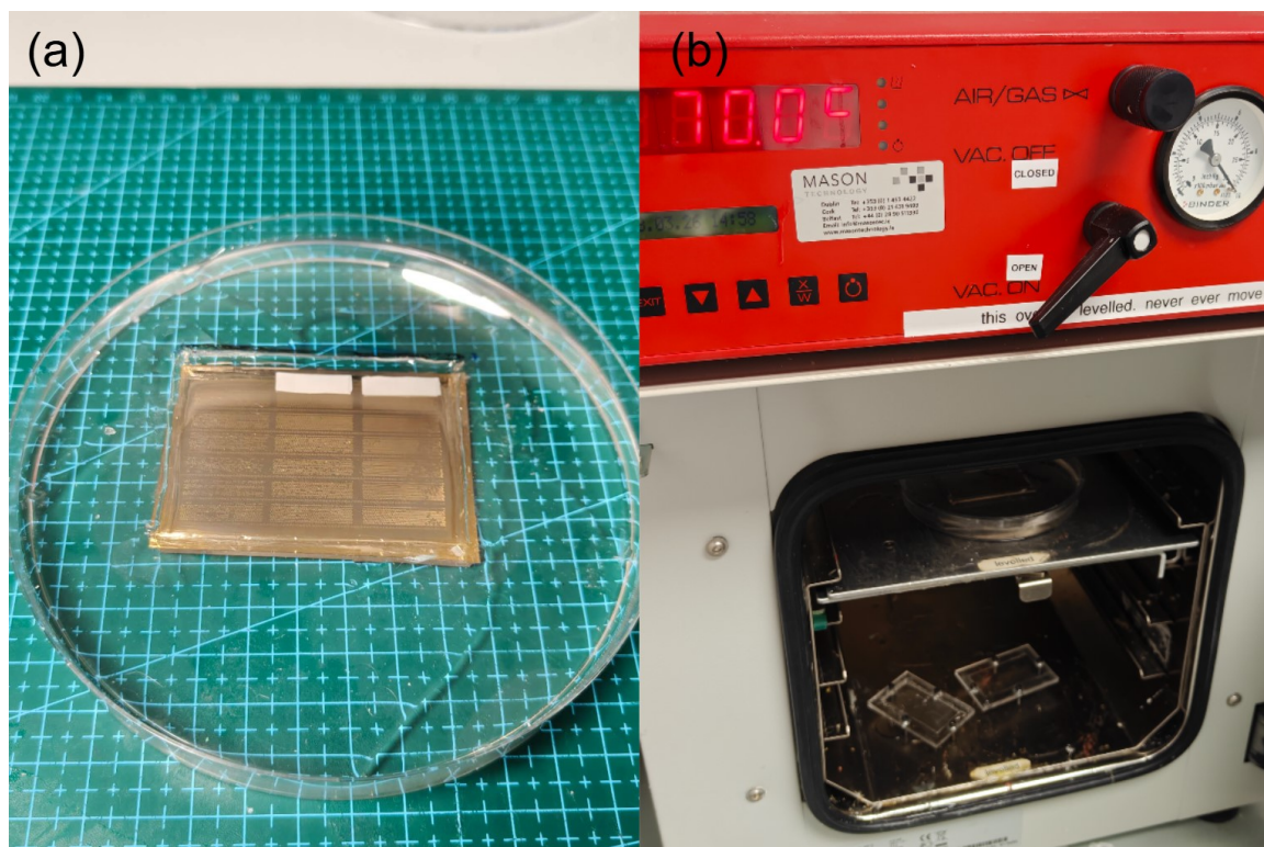
Figure 5.4: Preparation and thermal curing of the cast PDMS elastomer. (a) The nickel master mould assembly, containing the fresh, degassed PDMS casting layer, positioned on a petri dish carrier and placed on a cutting mat prior to insertion. (b) A standard laboratory convection oven (Mason) with its door open, set to the target temperature of 70.0°C. The prepared mould assembly is visible inside on the wire rack, ready for the 2.5-hour cross-linking process.
