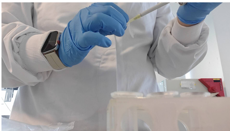
Figure 3.2: Use of personal protective equipment (PPE) during PDMS fabrication and chip handling. A lab coat and disposable nitrile gloves were worn whenever casting PDMS, cutting and demoulding chips, handling glass slides, or working with cleaning solvents.
