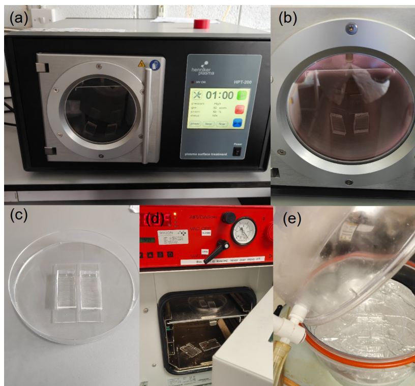
Figure 5.6: Sequential workflow for the interfacial bonding and preparation of the microfluidic chips. (a) The control panel of the Henniker Plasma HPT-200, displaying the batch processing parameters (60 s, 50% power). (b) The plasma chamber during active surface treatment, showing the simultaneous activation of two PDMS replicas and two glass slides. (c) The assembled microfluidic devices immediately following initial contact. (d) The bonded devices placed in a 70 °C convection oven for thermal stabilisation of the covalent siloxane network. (e) The fully assembled chips undergoing a 45-minute vacuum degassing cycle in a desiccator, preparing the bulk PDMS for passive fluidic priming.
